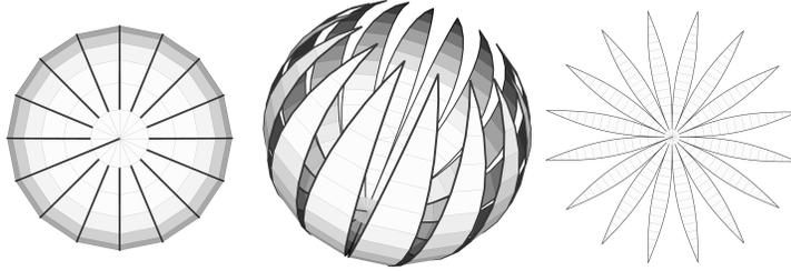
**Fig. 5.** Unfolding the sphere by cutting edges along geodesic curves.
